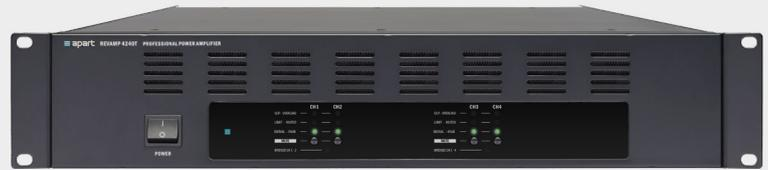
REVAMP4240T is a professional 4-channel digital power amplifiers with 4 x 240 watt output power @ 100 volt or @ 4 ohms. The unit is also bridgeable to 2 x 480 watts @ 100 volt (or @ 8 ohms). The unit incorporates a high reliability European designed Hypex amplification and power supply technology, outputs with efficient Class D output topology and output transformers.
